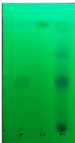
Figure 2. TLC profile of mangiferin with n -hexane and methanol extracts with ethyl acetate: formic acid: water (36:6:4) as the eluent, under UV \lambda_{254} nm (P = pure mangiferin, H = n -hexane extract, M = methanol extract)
