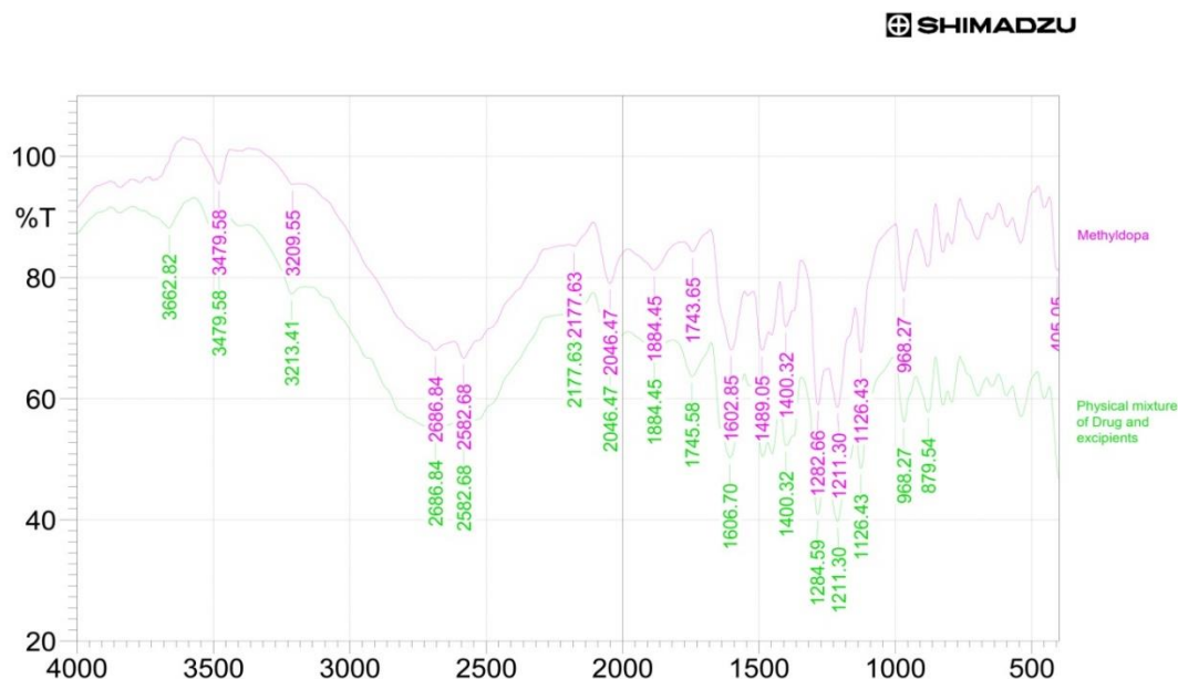
Figure3: FTIR Spectrum of physical mixture of Methyldopa, HPMC K 100 M and Carbopol 934
