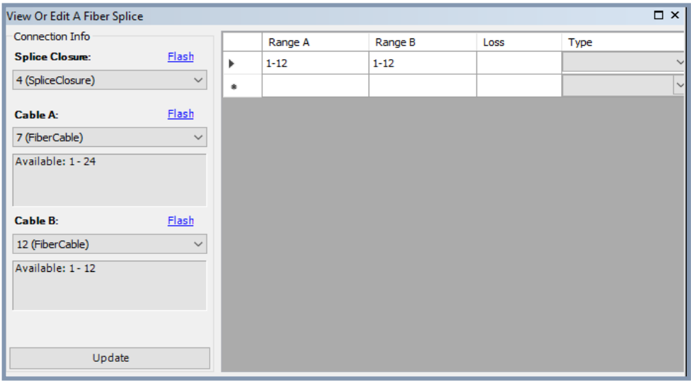
Figure (16) Edit Fiber Splice window. Source: Esri Fiber Editing Toolbar in Arc Map 10.7.1
